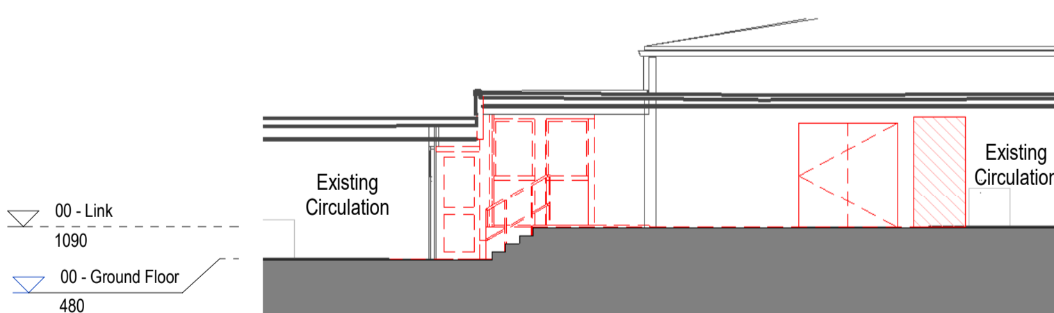
Phase 3 Section D-D Existing Link Scale: 1 : 100
